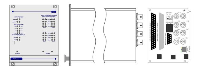
The **AMG3788BRN-DR-SF** is a rackmount eight channel video receive unit designed to receive up to 8 video signals from a single fibre optical fibre ring with Dual Redundant operation. It also provides 9 bi-directional data/audio channels via a low speed data interface. Eight of the data/audio channel interfaces, whether RS-232, RS-422, RS-485, 20mA, TTL, Contact Closure, Lonworks or Audio, are defined at manufacture by the addition of daughter boards fitted onto the Data Expansion Board B.
