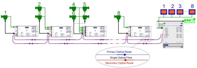
If a fibre link is broken, operation of the ring continues by making use of the secondary optical fibre route as below:
