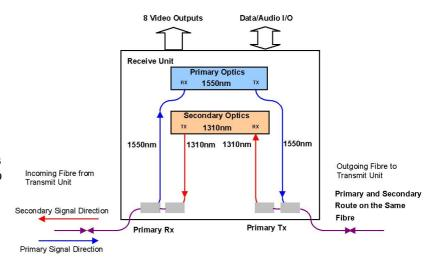
As each unit regenerates the optical signal, the optical dynamic range between each optically connected node is 17dB.
